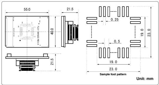
Figure 4.2 External dimensions of FLX-144NSD
